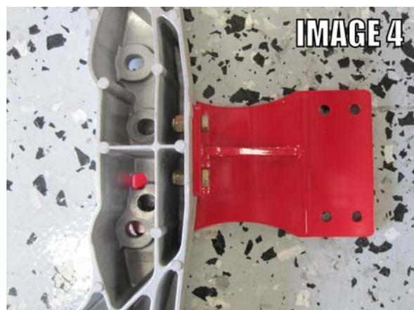
8. Using the supplied 3/8" x 1" bolts, washers and nuts, bolt the BMR mounting bracket to the OE crossmember as shown in **Image 4**.
