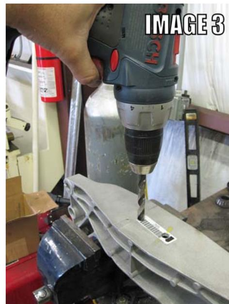
7. Remove the BMR mounting bracket and drill the two holes into the factory cross-member as shown in **Image 3**.
