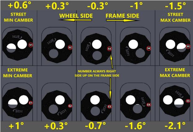
**NOTE**: If more or less camber is desired, use a different flat on the lockout to move the control arm **IN** for more positive camber or **OUT** for more negative camber (see table) Caster can also be adjusted by staggering the lockouts on the lower control arm. If more fine adjustments are needed, use BMR part number **WAK561**
