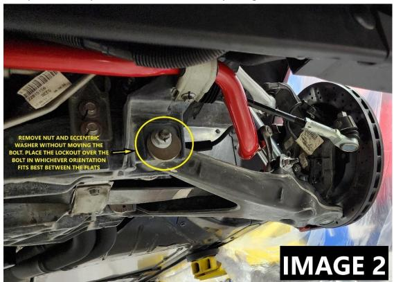
4. After you have selected the setting that best suits your application, remove the eccentric bolt and install the matching lockout for the other side of each mount and bolt it together
