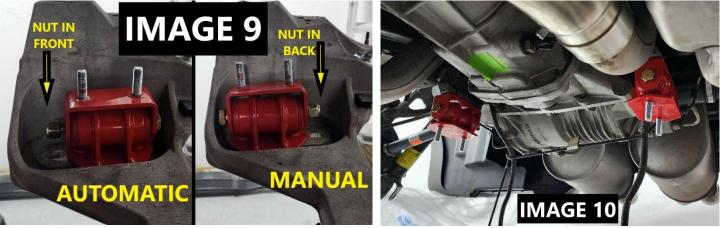
**NOTE:** When installing the transaxle mounts, be sure the bolt head is on the appropriate side that offers the most clearance for the nut. i.e. if the mount is in the front holes, the bolt should go in through the front. If the mount is in the rear holes, the bolt should go in through the rear. **IMAGE 9**
