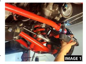
3. Remove the four (4) bolts holding the rear sway bar saddles on the frame with a ½" socket. **IMAGE 1**
