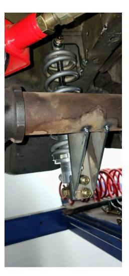
**NOTE:** Refer to your coilover manufacturer for the recommended installed height. For the recommended Viking C209-W shock, it should measure 13.75-15" eyelet to eyelet at ride height.
