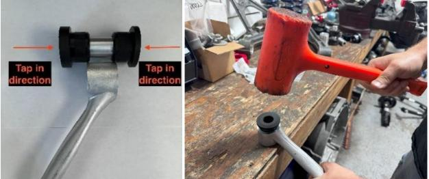
25. According to the figure, tap the bushings into the control arms using a rubber mallet. **NOTE:** Make sure the correct bushing part number is tapped in based on the location. Some bushings have the same outer diameter but different flange thickness lengths. The outer bushings will have a thicker flange thickness than the inner bushings.
