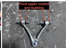
36. According to the figure, tap the bushings into the control arms using a rubber mallet.
