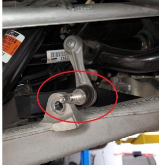
6. Using a 21mm socket and wrench, loosen the inner bolts of the lower control arm
