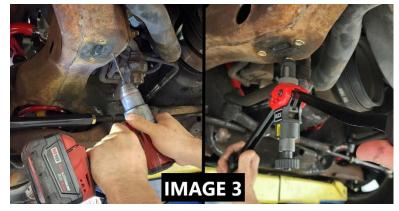
**NOTE:** 5 Rivet nuts are included so the four threaded holes for the stock sway bar mount can be riv-nutted for strength. These holes will also need to be drilled to 7/16"
