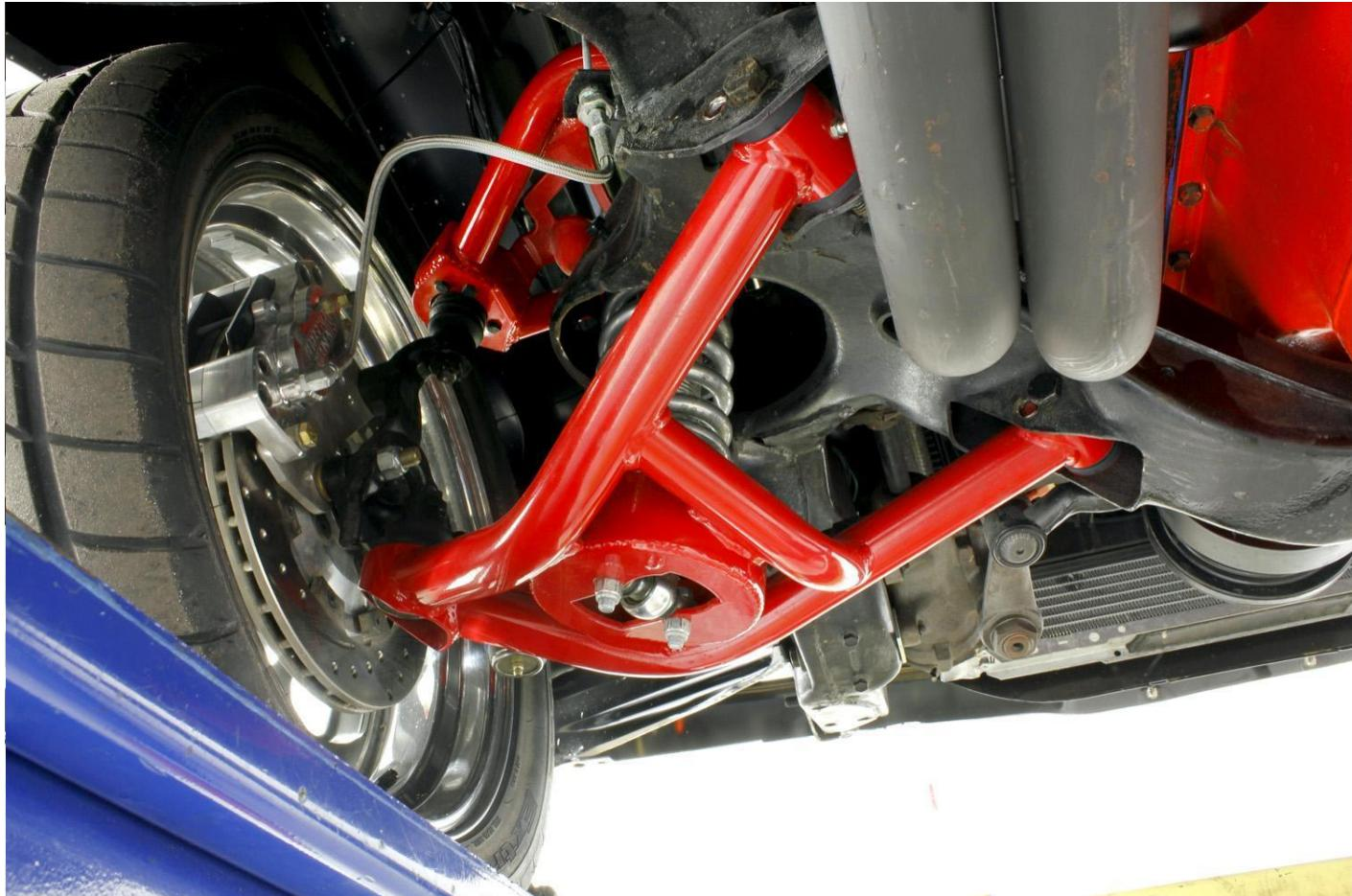
BMR A-arms have improved geometry built into the A-arms. Your BMR A-arms have an additional 2 degrees of positive caster built into the arm which will affect your alignment. It is necessary to have the vehicle re-aligned after this installation. BMR recommends the following alignment specifications:
