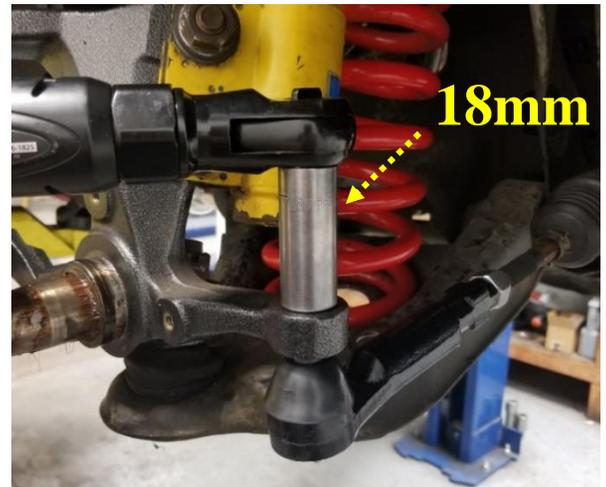
10. Use a jack and support the lower control arm. This is **critical** because the spring is *pre-loaded* and you could experience *explosive decompression* if the arm is not supported when you remove the shock from the spindle.
